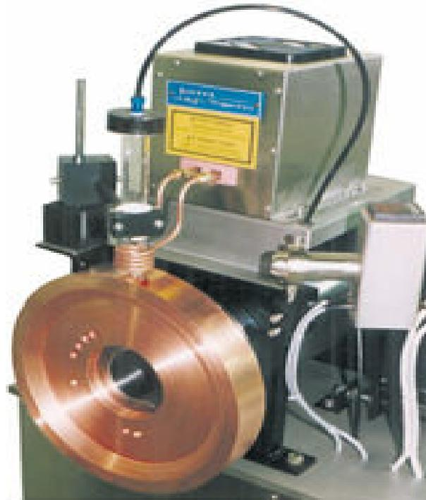
Fig. 4.2 Melt-spinning Mechine
