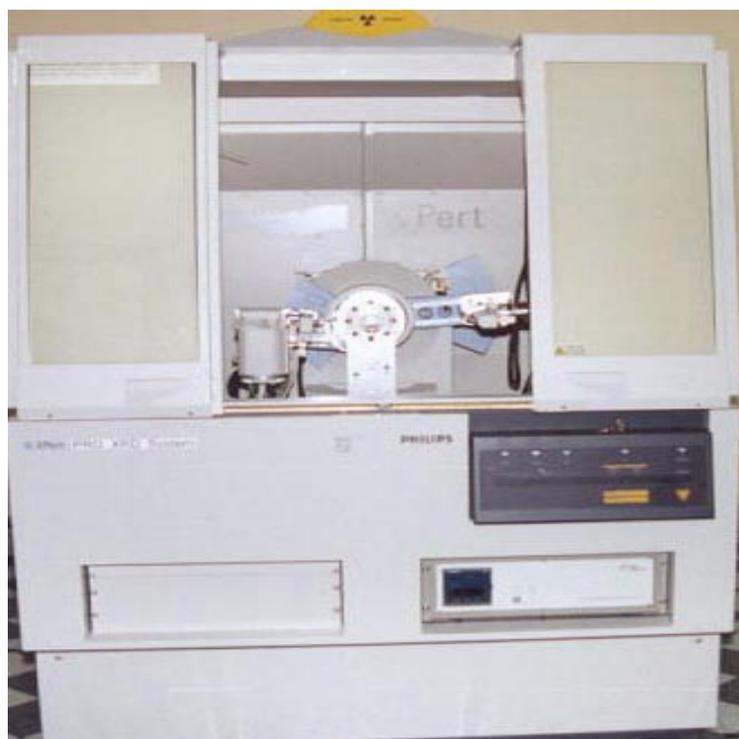
Fig.4.8 A PHILIPS PW3040 X'Pert PRO X-ray diffractometer.
