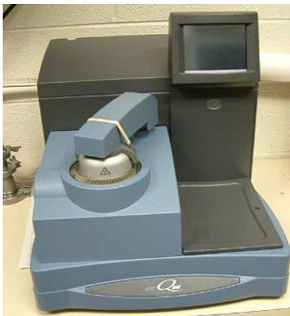
Fig. 4.4 Differential Scanning Calorimeter (TA Instruments Q100).
