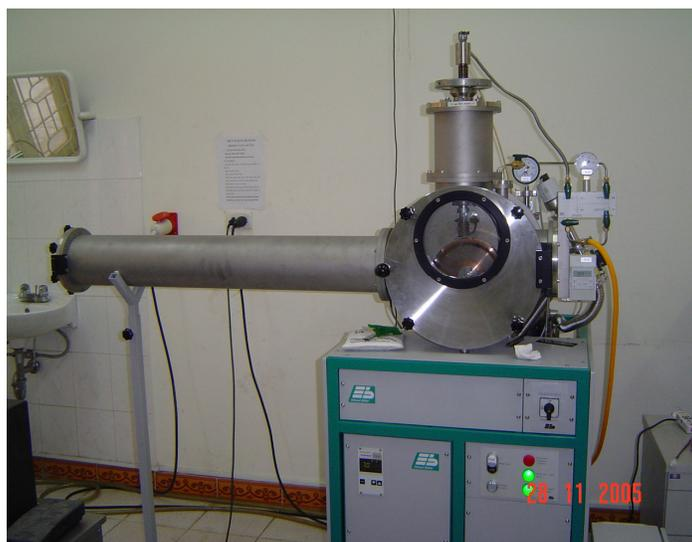
Fig.4.1 Vacuum arc melting machine
